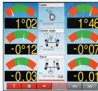
Easy-to-read rear meter provides caster, camber, and toe, all on one screen.
