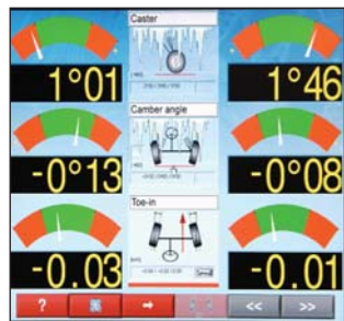
Front meter screen with frozen readings - freezes the readings to allow the technician to lift or move the vehicle then make the readings live again.
